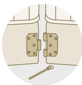
Boxspring fastened to the head of the bed with a pivot
